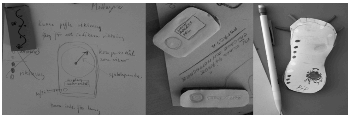
Figure 3. To the left a paper prototype of the receiver inspired by a compass and a sender inside a piece of jewellery; in the middle a sender with a nametag and a button; to the right, a receiver made of paper, a flower foam brick and flower sticks.
