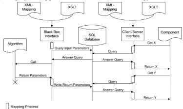
Figure 3: Interaction Scheme for Automatically Generated Interfaces
