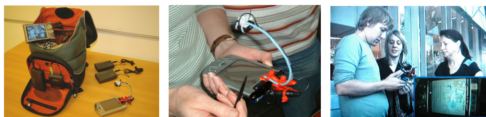
Figure 8: The mobile field laboratory (left), wireless micro camera mounted on mobile device (middle) and the video recording of participants, interviewer and physical surroundings with inserted close-up of mobile device interface (right)
