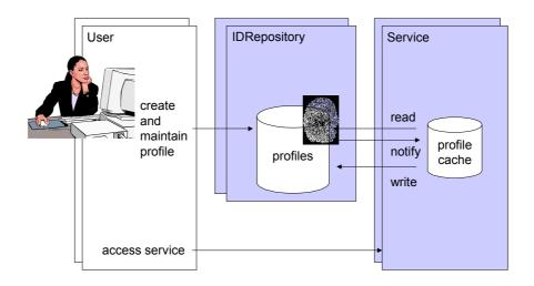
Figure 2: Identity Management Architecture Components.
