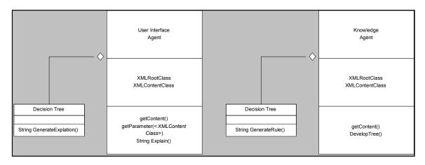
Figure 2. Class Diagram Showing the User Interface and Knowledge Agent Details
