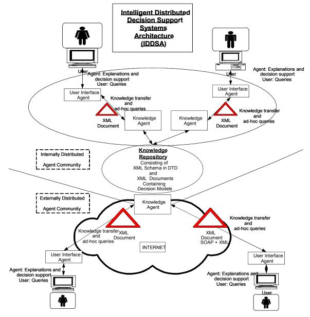
Figure 3. Intelligent Distributed Decision Support Systems Architecture (IDDSA)
