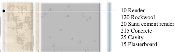
Fig. 3 – Externally Insulated Solid Wall Case Study 2
