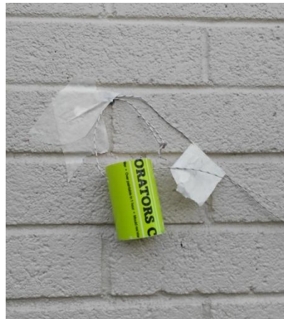
Fig. 13 – External thermocouples fixed
