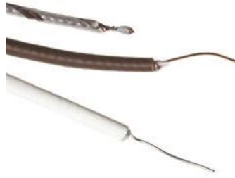
Fig. 8 –T type thermocouples
