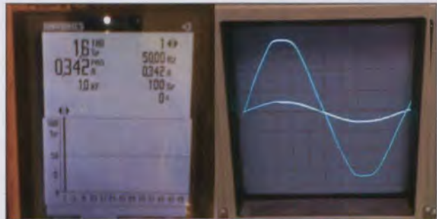
Figures 8 and 9: two GLS lamps in parallel
