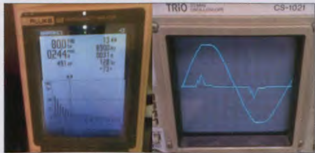
Figures 10 and 11: two CFLs in parallel
