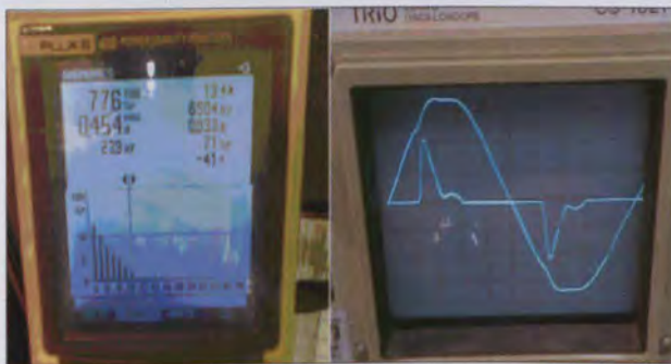
Figures 14 and 15: six CFLs in parallel
