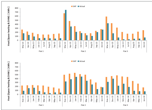
Figure 8: SAP and actual heating energy use for the three apartments for March 2013 to the end of June 2014.
