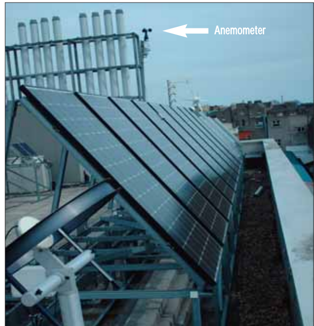
Figure 7: Anemometer mounted on bracket over PV array on roof of DIT Kevin St Campus renewable research facility
