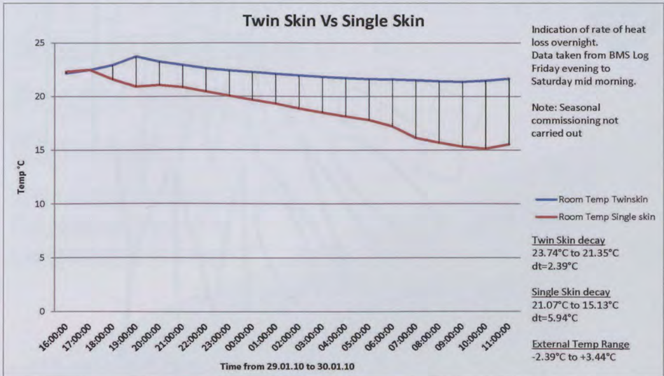
Fig. 1.7: Twin skin vs single skin. Courtroom versus office area
