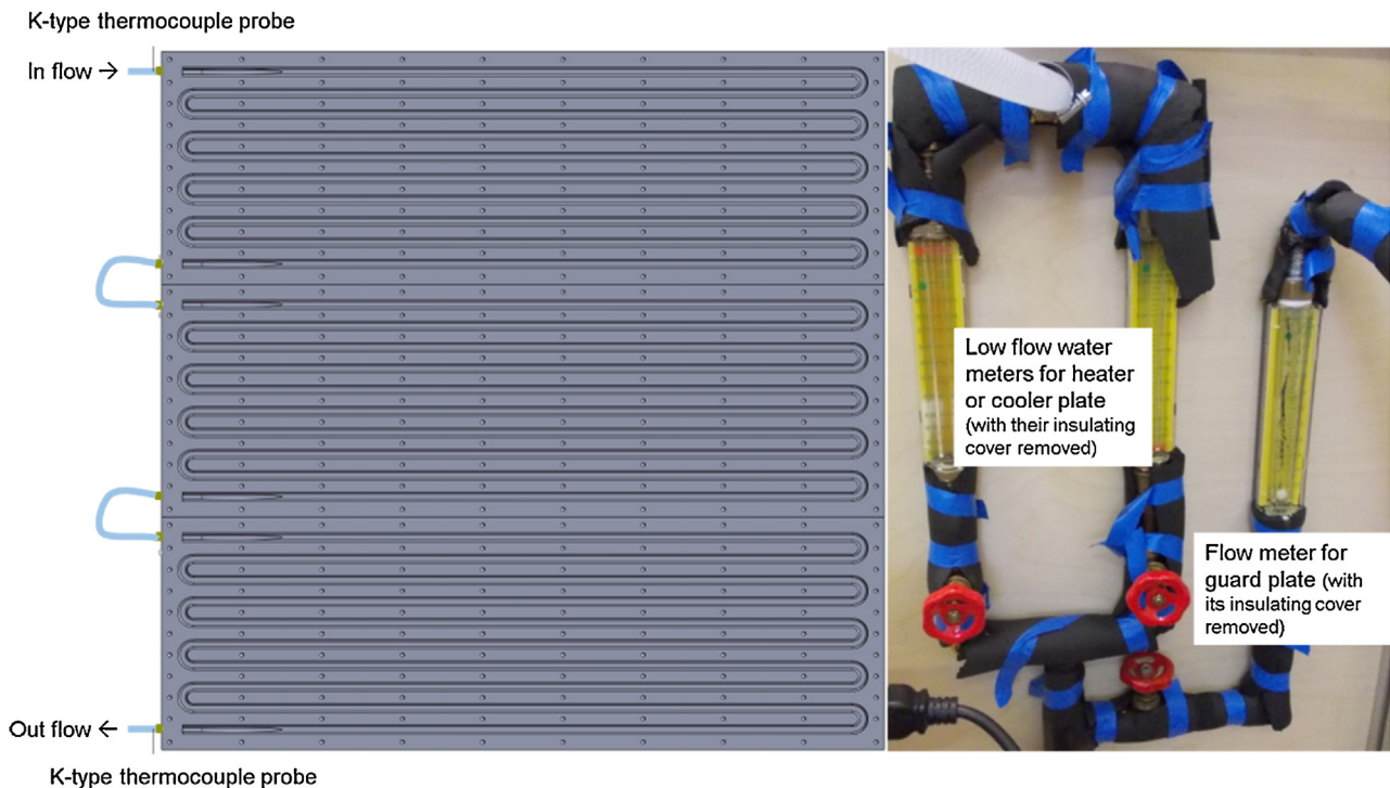
Fig. 5. Internal channels of plates showing the location of temperature measurement on in and out flow, and flow meters to measure flow to the heater/cooler plate and guard plate.
