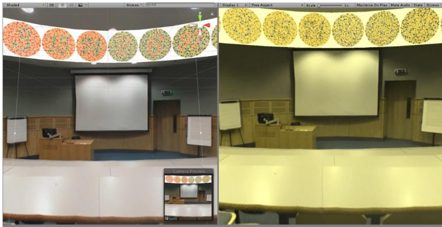
Figure 2. Unaltered 360 photography of a lecture hall (left) and the view of the same image rendered by the virtual camera with a deuteranopia filter applied (right). Ishihara plates used for validation are visible at the top of each image.
