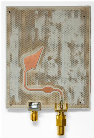
Fig. 7. Photograph of the optimized antenna.
