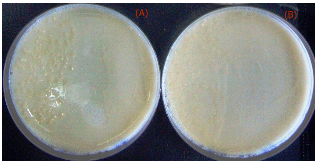
Fig 3.14 Petri dishes of (a) Sigma-Aldrich ZnS agar plate inoculated with E. coli and S. aureus exposed to light and (b) Sigma-Aldrich ZnS agar plate inoculated with E. coli and S. aureus not exposed to light.
