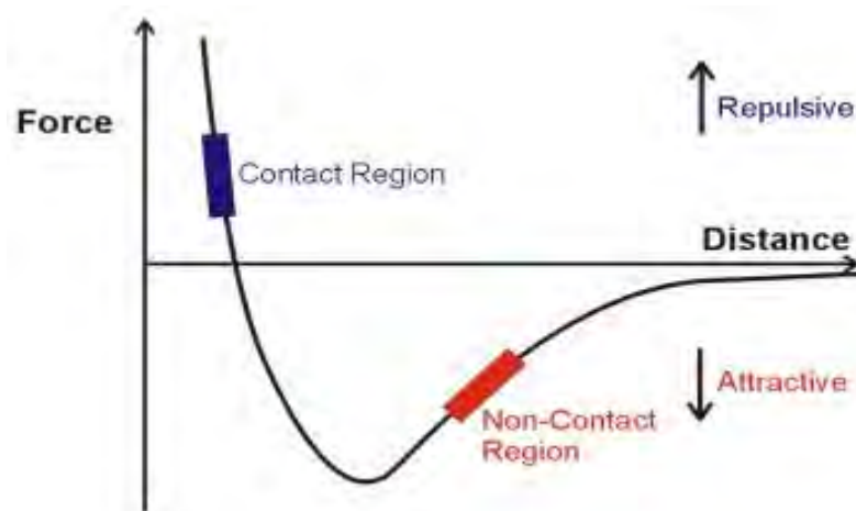
Figure 3.18 The region where the contact and non contact mode can be operated [36]
