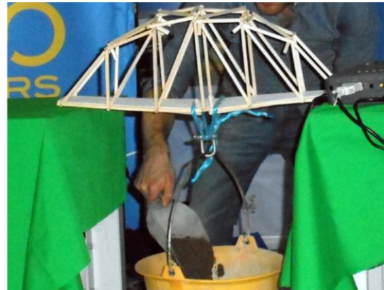
Fig. 4. Testing of balsawood models.
