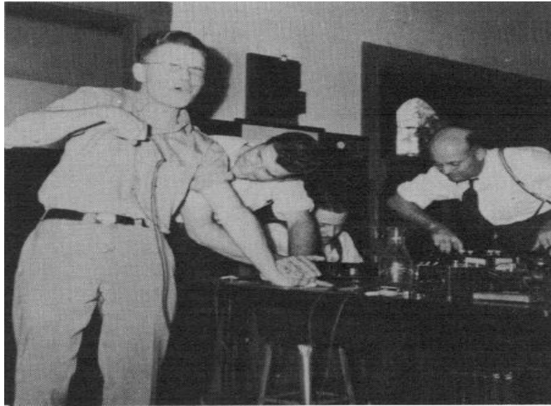
Figure 2-4 Subject under investigation to determine the let go threshold [49]
