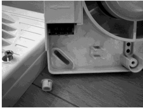
Figure 3-3 An enclosure of an extractor fan preventing direct contact of live terminals
