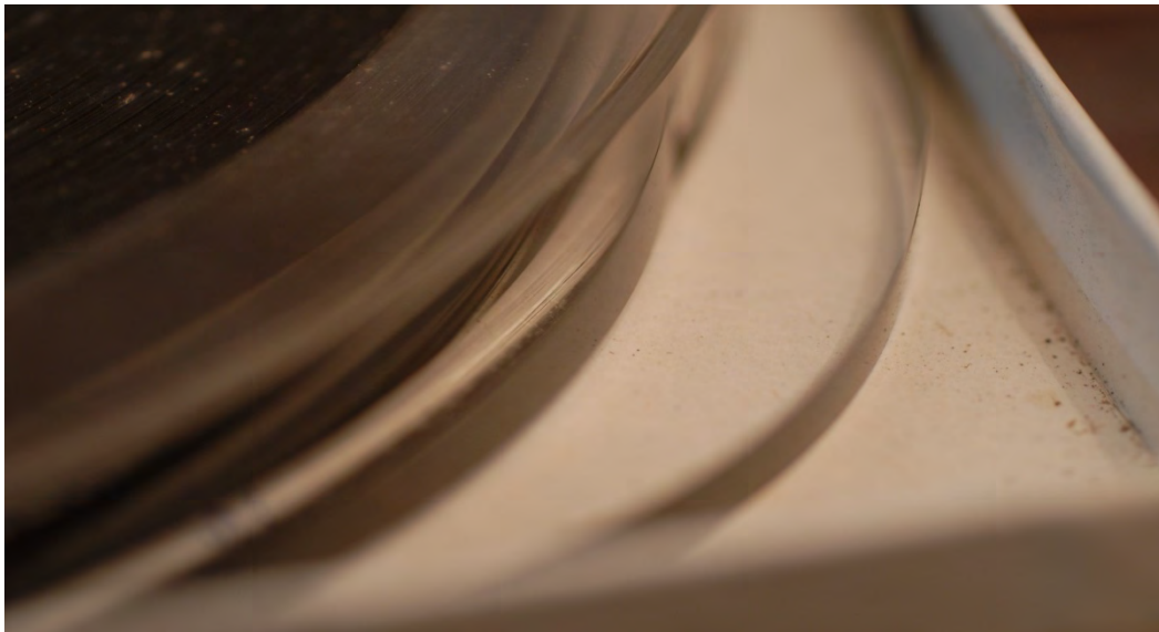
Figure 2:17: Example of worn tape (top); Magnetic dust gathers in the corner (bottom).
