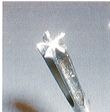
Fig. 3.3. Molar-end cutting implement.
