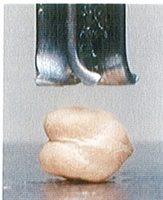
Fig. 3.4. Sample orientation during compression testing.
