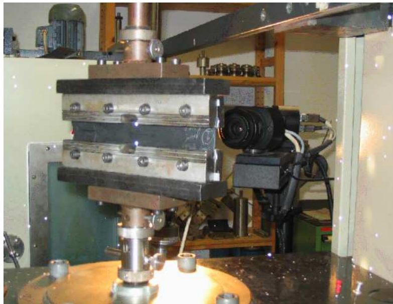
Figure 3.6: ICP system and experimental set up with a planar specimen clamped at 0% integral strain.
