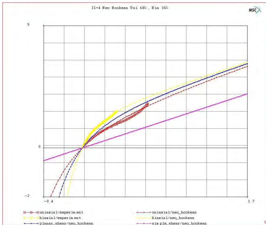
Figure A.8.1: Neo Hookean material model
