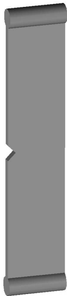
Figure 3.5: SEN specimen with ribs to aid clamping
