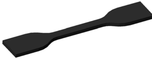
Figure 3.1: S2 sample as used for tensile stress strain measurements
