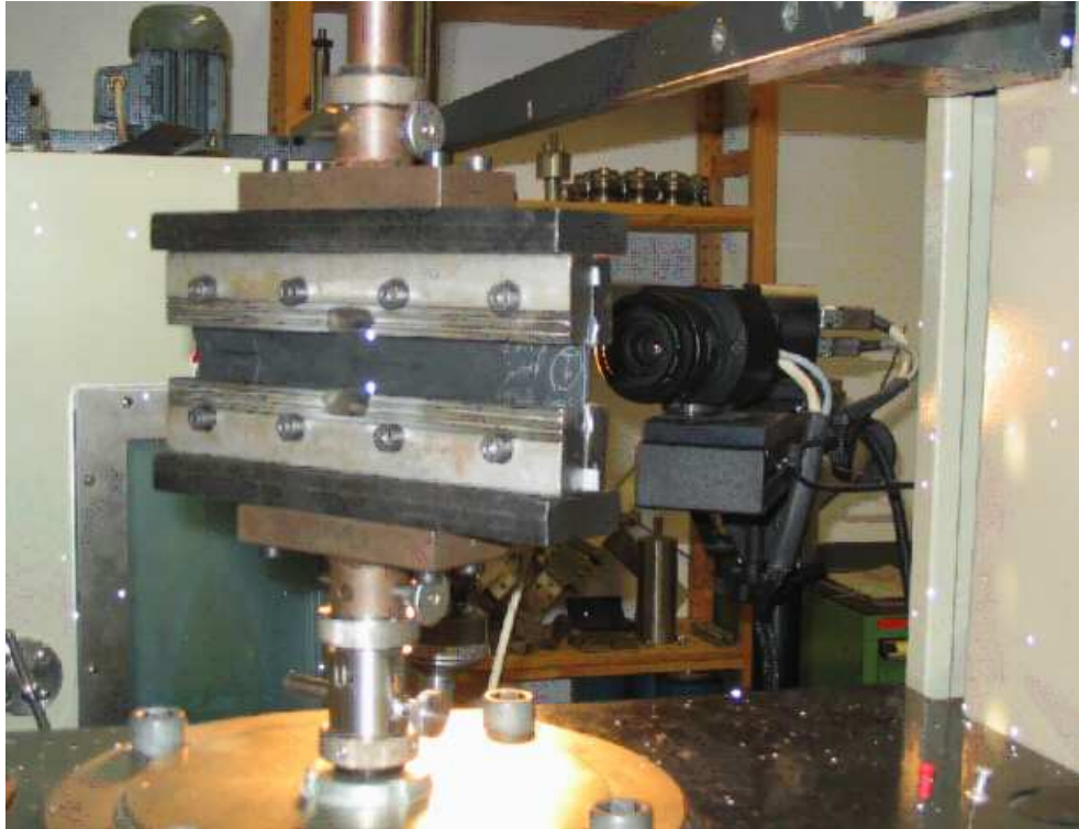
Figure 4.12: ICP system and experimental set up with planar specimen clamped at zero strain
