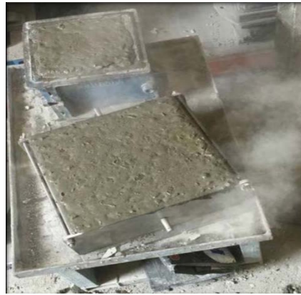
Figure 3 Schematic of the concrete slab cast
