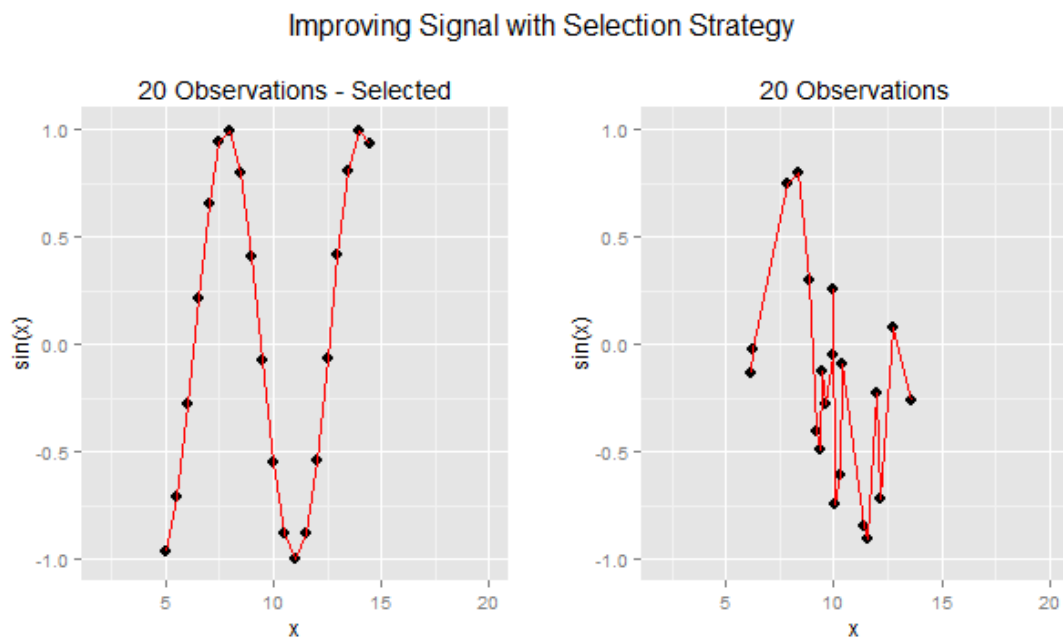
Figure 2 The sine wave function is apparent even with a small number of observations when these observations are carefully chosen. The figure on the left selects only observations with no noise, evenly distributed across the x axis. The figure on the right relies on random sampling from a normal distribution,
