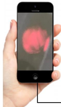
b). Camera colour sensitive profile before exposure to analyte
