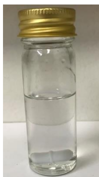
Figure 6. 6.Cellulose acetate and polyethylene (CA/PEG) blended solution
