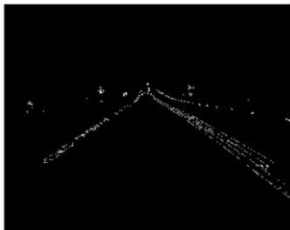
Figure 3: (b) Sobel edge map of test image
