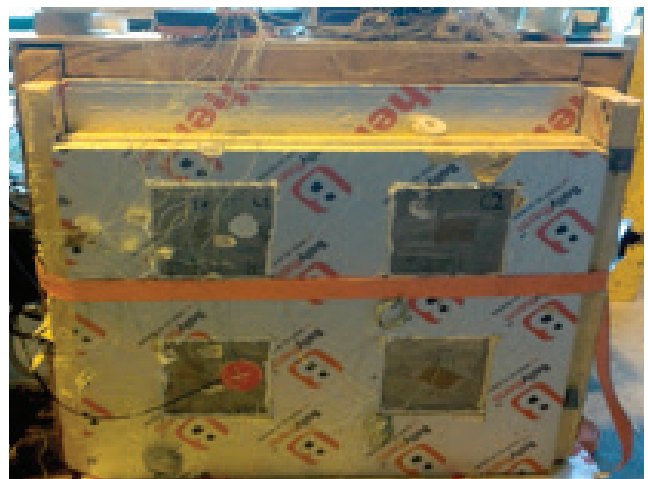
Figure 6. Concrete samples placed in the hot plate rig
