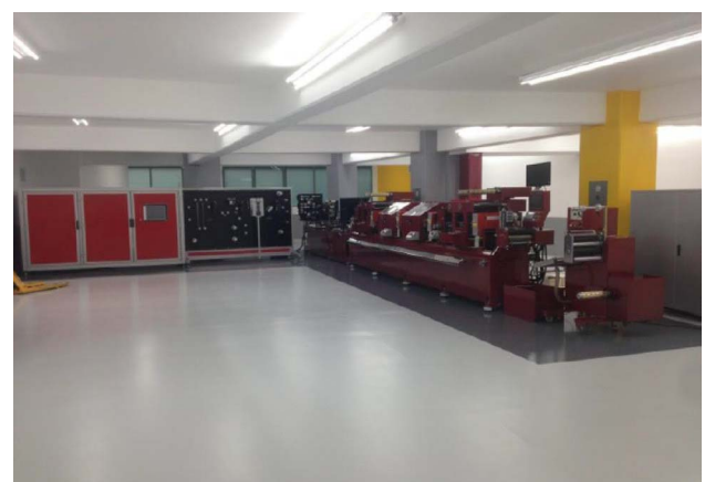
Fig. 3. Left side, Optrace serialized hologram production machine 6 \text{ m} \times 1.75 \text{ m} \times 1.8 \text{ m} . The user's web is at 90^\circ on the right.
