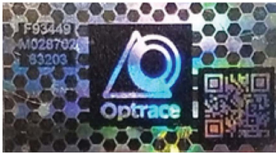
Fig. 7. Alphanumeric code (upper left) and the mobile telephone scannable QR code (lower right), are both holographic and unique to the reflection hologram (40 mm × 20 mm) shown. The other features, if required, may be repeated in many holograms.
