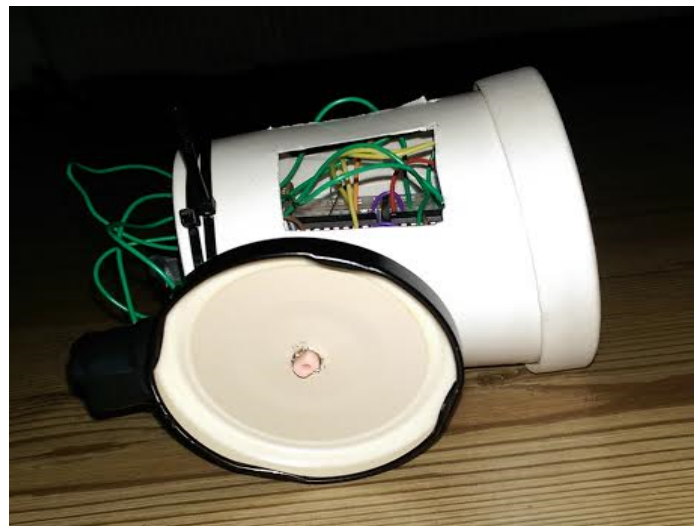
Figure 1. Sample Robot. This figure illustrates an example robot constructed with a take-away soup cup chassis and jam jar lid wheels.
