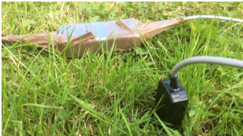
Figure 22: Soil Moisture Sensor and Microcontroller in-situ
