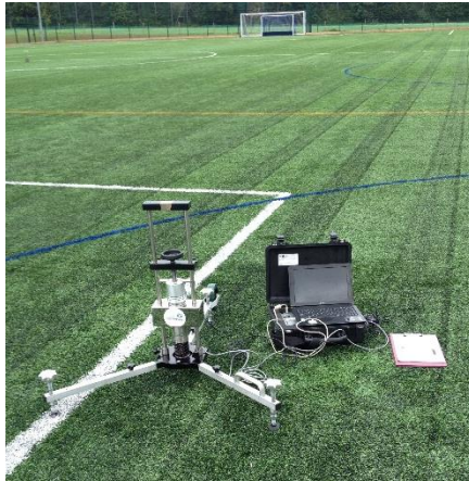
Figure 8: Shock absorption apparatus with a Piezo-resistive accelerometer
