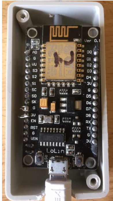
Figure 24: ESP8266 Microcontroller in plastic housing
