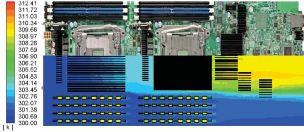
Figure 1: Intel server board S2600TP and sample CFD simulated temperature distribution (air-cooled situation)
