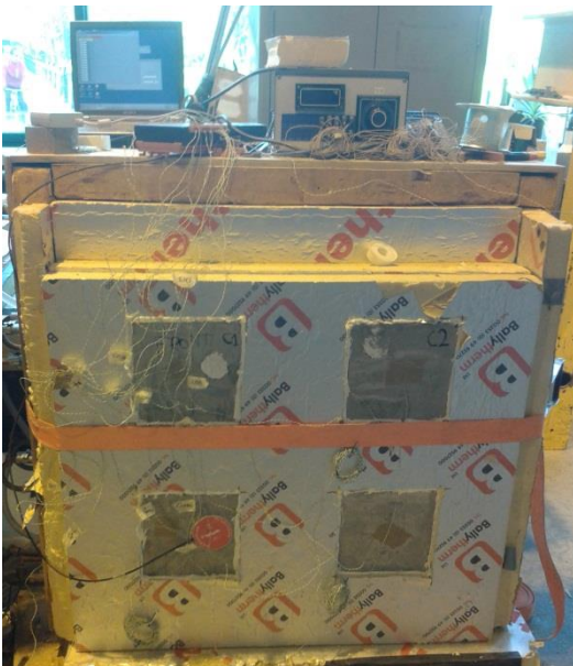
Figure 5. Concrete samples placed in the hot plate rig
