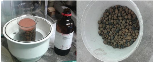
Figure 2. Manufacture of the aggregate/PCM composite
