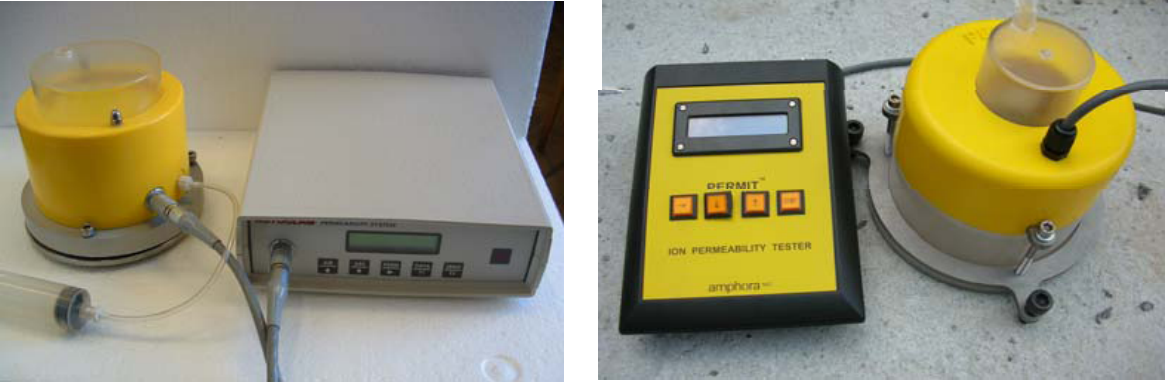
(a) Autoclam permeability apparatus [9] (b) Permit chloride migration ion diffusion apparatus [10,11]
