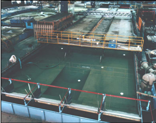
Figure 4-1 Aerial view of FCF (Phase C straight compound channel test in progress)
