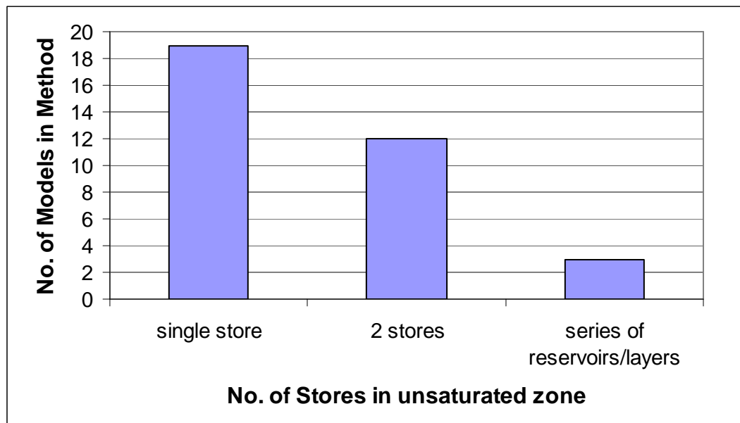
Figure 19 Representation of unsaturated zone in conceptual models
