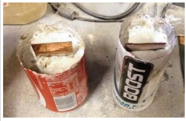
Figure 6: Battery housed in a metal can.
