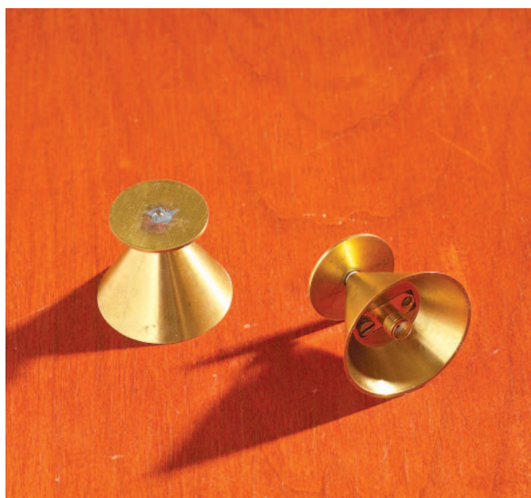
Figure 2. The discone antenna developed at I 2 R.
