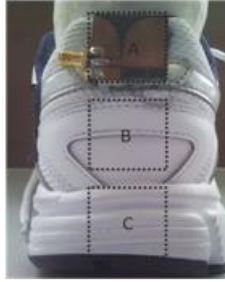
Fig. 12. Top (A), middle (B) and bottom (C) position of the Vivaldi antenna.
