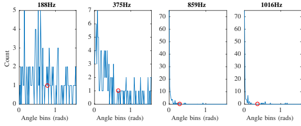
Fig. 4. Illustrating bi-modality: consider a mixture of a violin and speech in four frequencies in TF, e.g. 188, 375, 859 and 1016 Hz. Speech dominates the mixture at 188 and 375 Hz. The violin dominates the mixture at 859 and 1016 Hz. The violin histograms have their highest count at 0 radians. When the speech is dominant the histogram exhibits two concentrations. The higher (radian) concentration corresponds to the speech energy, the lower (radian) concentration corresponds to the violin. The selected threshold (red dot) is lower when speech dominates.
