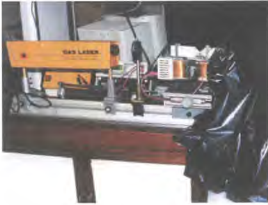
Figure 2. Apparatus showing laser (left) followed by polariser and magnetic poles (right)
