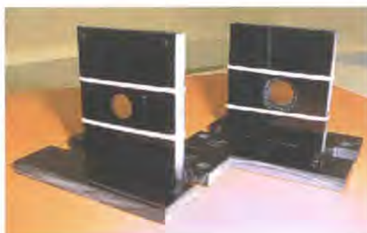
Figure 1. Novel transmission measurement cell constructed for this project
