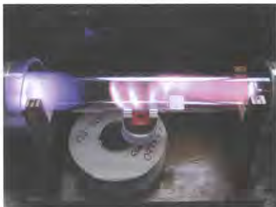
Figure 1. Atmospheric plasma used in this work showing striations in this case in the presence of a magnetic field.
