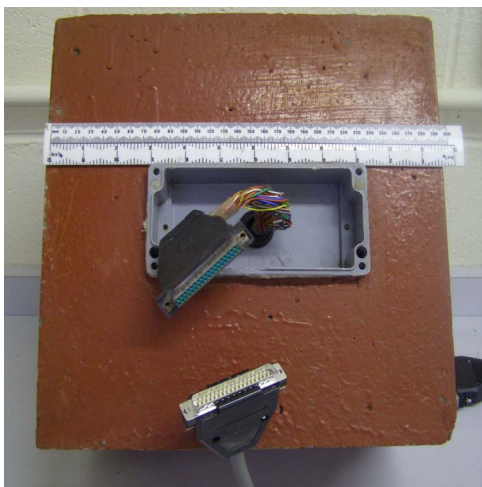
Fig. 2. Schematic diagram of (a) embedded array and cable termination; (b) GRP enclosure and lead termination at a 37-pin D connector
