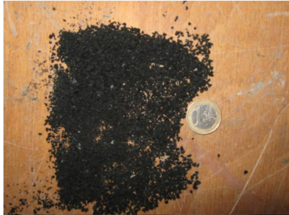
Figure 3 3mm crumb rubber particle used in concrete
