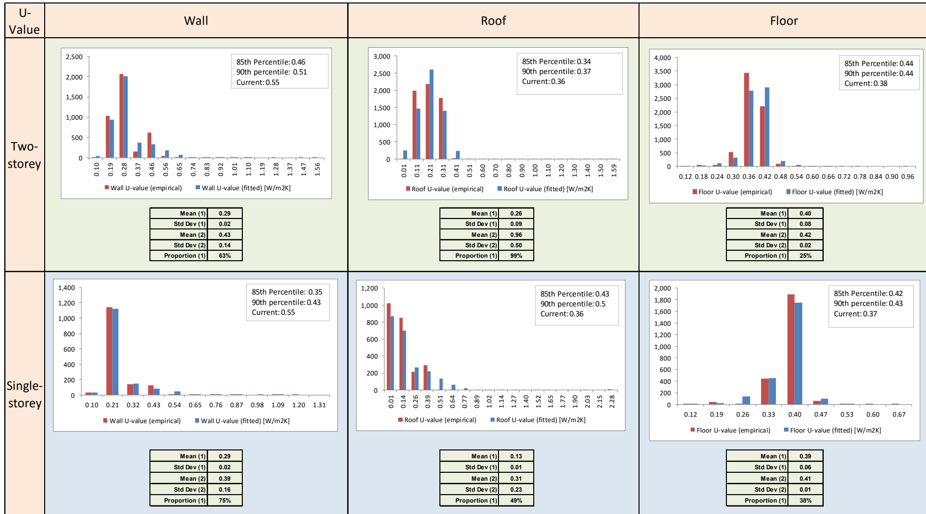
Figure C9 Statistical analysis of dwelling envelope thermal frequency distributions for dwellings constructed between 2000 and 2004
