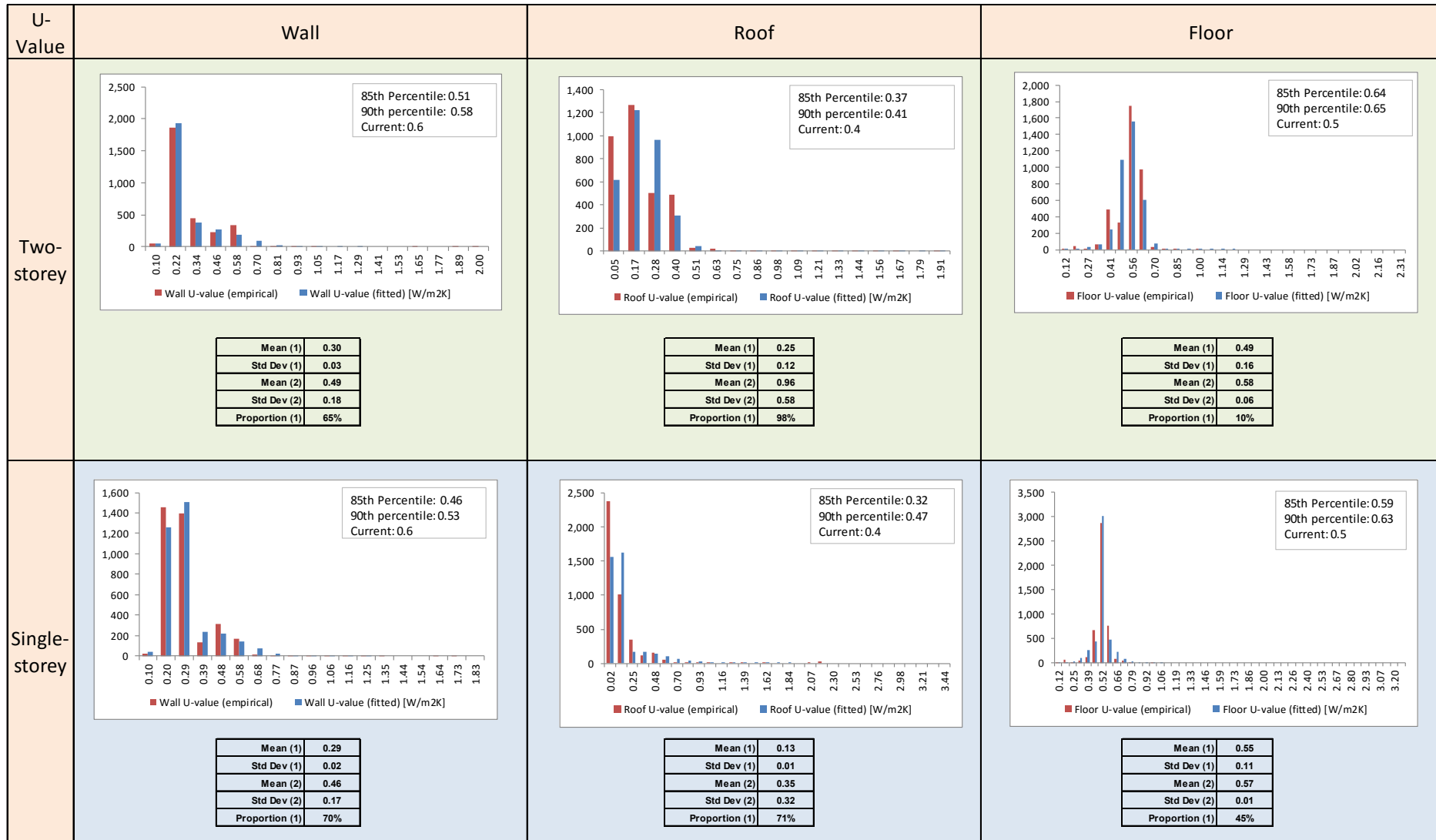
Figure C7 Statistical analysis of dwelling envelope thermal frequency distributions for dwellings constructed between 1983 and 1993
