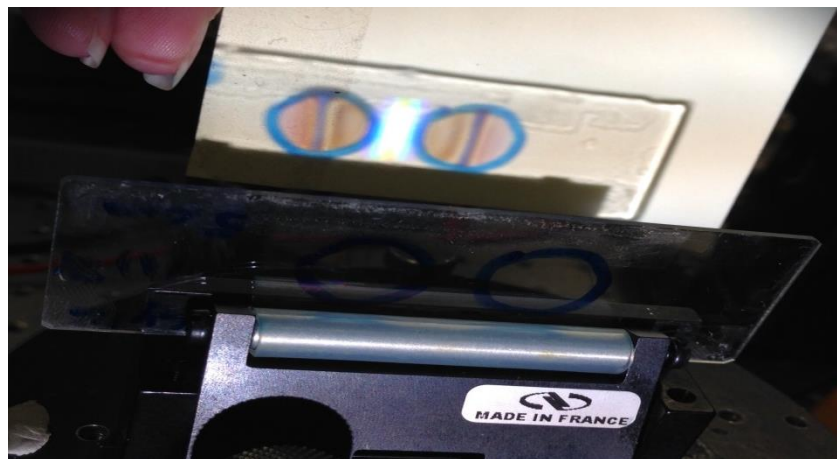
Figure 6-11 Photo taken through holographic lenses recorded in acrylamide photopolymer reconstructed with solar simulator light source the central band of white is the diffracted, focussed light diverted by the two gratings , overlapping at the appropriate position.
