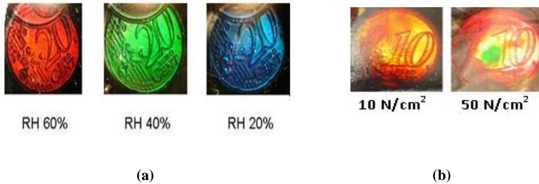
Figure 1-6 a) The IEO holographic humidity sensor as the relative humidity is increased from 20-60 % and b) The IEO holographic pressure sensor as the pressure is increased from 10 N/cm 2 -50 N/cm 2
