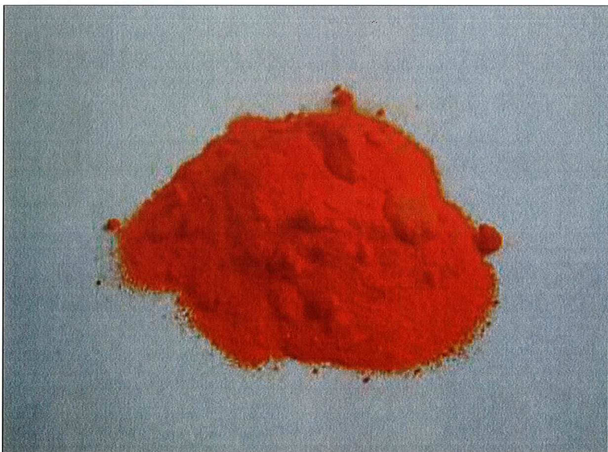
Figure 1.1. Potassium Dichromate (molecular formula K_2Cr_2O_7 ) has a red-orange crystalline solid appearance. As with other Cr (VI) products, potassium dichromate is carcinogenic. It is a powerful oxidizing agent and is the preferred compound for cleaning laboratory glassware of any possible organics ( http://upload.wikimedia.org/wikipedia/commons/2/23/Potassium_dichromate.jpg ).
