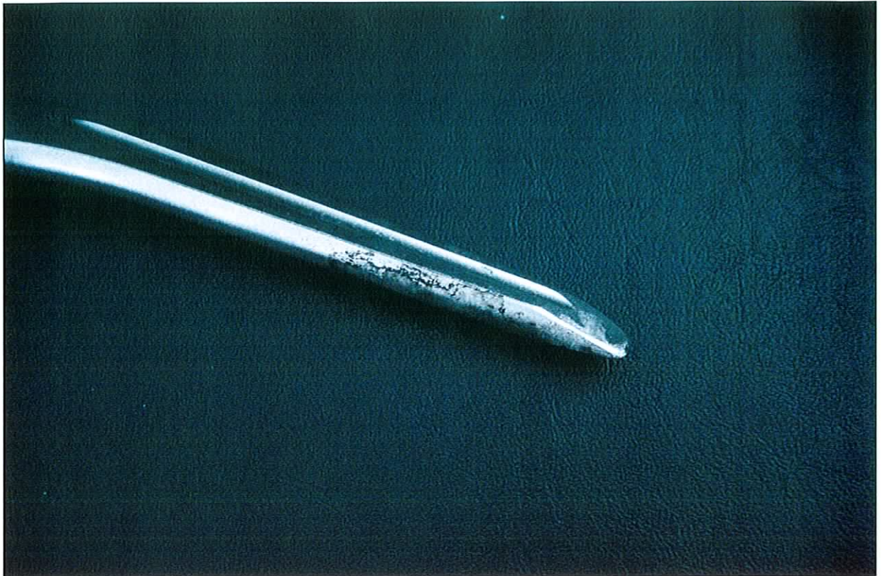
Figure 1.7. Metal prosthesis showing corrosion on the socket.
