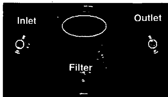
Figure 8.17 2D Harmonic image showing the placement of the 3 ROIs, inlet vessel, perfused area in dialysis filter and outlet vessel
