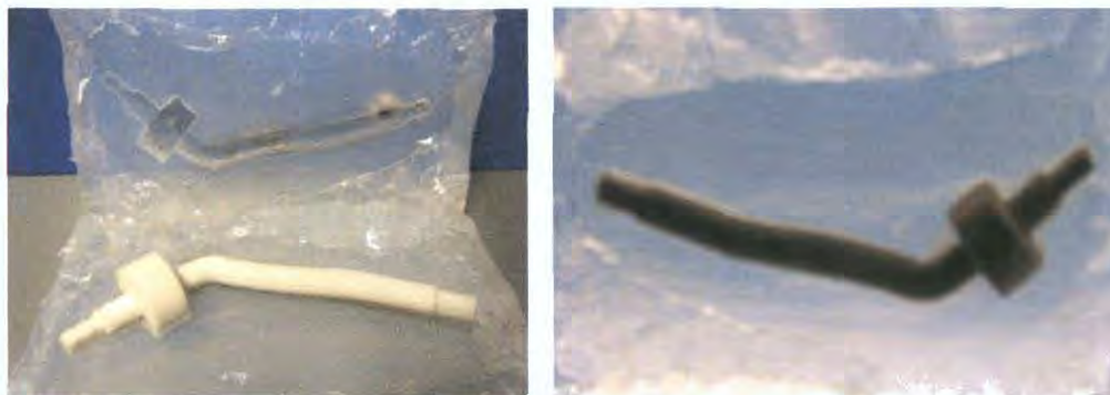
Figure 3.5 Development of soft tool for renal artery lumen
