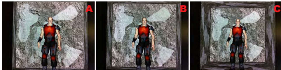
Figure 3.7: Boxing only: As the user moves closer or further away from the display the scene is updated to reflect the change in depth from the user's perspective. A: Viewed from far away, the further the viewer is at the shallower the depth of the box. B: Viewer is closer the 2D display, more of the box's interior is becoming visible. C: Viewer is even closer to the 2D display and they have a clear view of the box's interior walls at this point due to increased depth.
