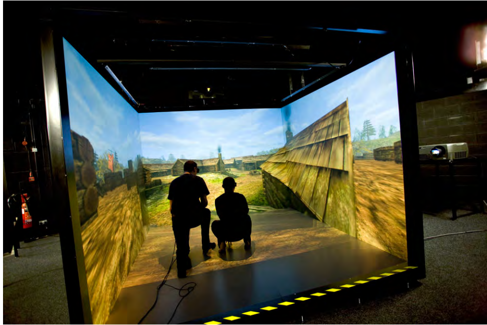
Figure 2.1: CAVE system in operation with two occupants.
