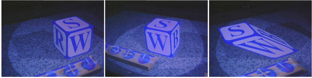
Figure 1.6: The image to the left is of the rendered scene on the Workbench for a user’s perspective who is standing on the left side of the table. The image in the centre is from a user’s perspective who is standing to the right side. The image on the right is the view that a user standing on the left side of the table would see if the 3D scene was generated for the perspective of a user standing to the right of the Workbench and it suffers from lateral foreshortening. Even though the image on the Workbench is the same in both the centre and right images, the cube appears sheared to the non-tracked user.
