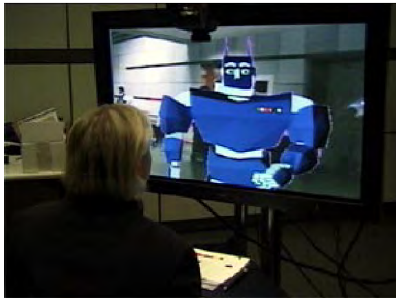
Figure 1.2: A user interacting with MACK (Cassell et al. , 2002), the scene behind the 2D display is rendered to the screen to make it look as if MACK is standing within the user’s environment.
