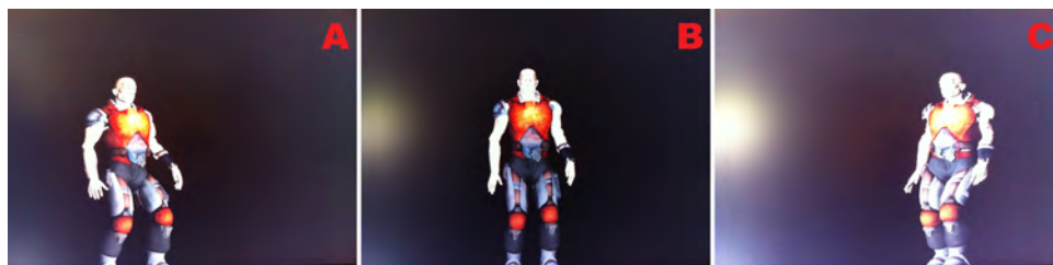
Figure 3.6: Stretching only : As the virtual camera moves the scene is stretched to compensate for lateral foreshortening. A : Viewed from far left. B : Viewed from sweet spot. C : Viewed from far right.
