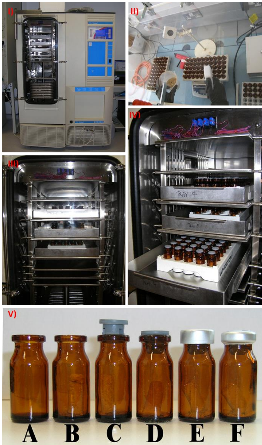
Figure 5-11: Pictures showing the various steps in the freeze drying process, I) Virtis 50XL instrument, II) dispensing freeze dried materials inside modified glove box, III) dispensed materials in freeze drier with shelves contracted to push lyophilisation stoppers into place IV) sealed aliquots of freeze dried materials and V) various stages of materials being dispensed with empty containers (A) to sealed and crimp capped aliquots (F).
