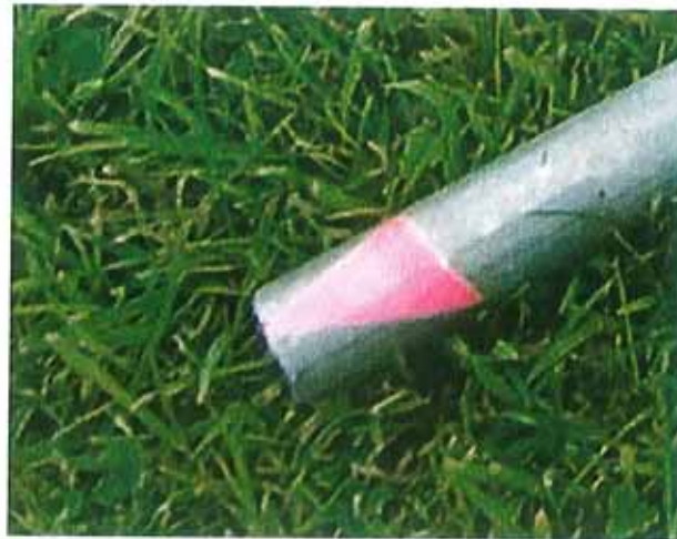
Figure 7.8. Target at end of pipe.
