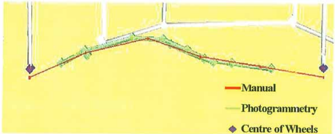
Figure 4 PhotoModeler model of Jaguar XJ with manual measurements shown.
