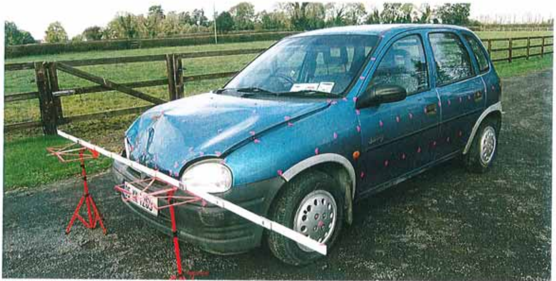
Figure 8.7 Opel Corsa (with Bumper, hiding extent of damage)
