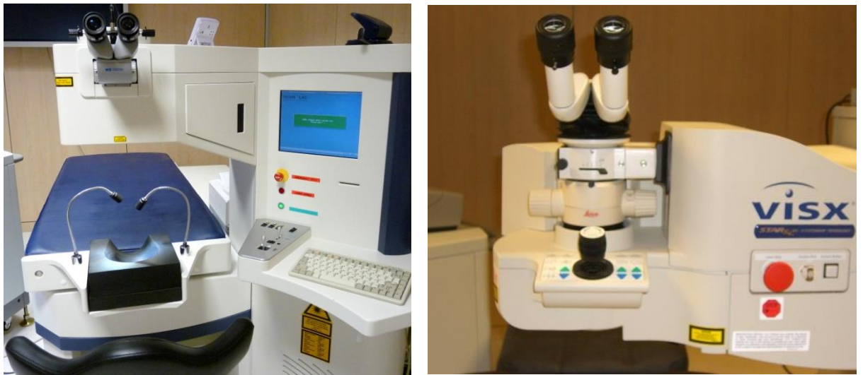
Figure 2-8: Technolas 217z (left) and Visx Star S4 (right) Excimer laser systems
