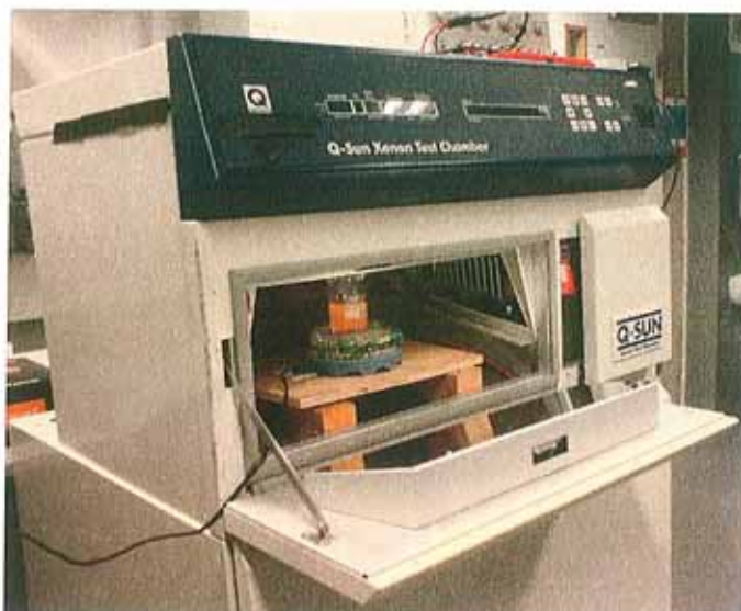
Figure 2.2: Picture of the Q-sun solar chamber used for the photocatalytic light irradiation experiments.
