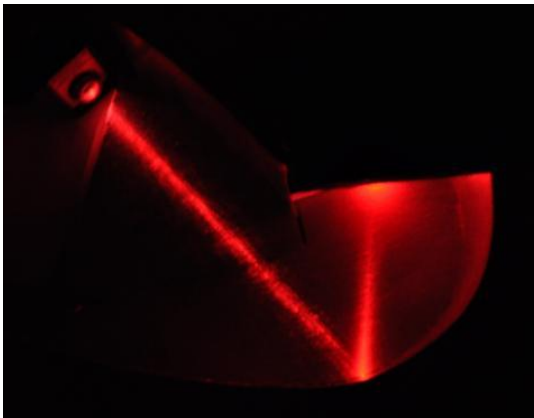
Figure 3.13: (c) Test-2 Laser ray on circular reflector of CTAH
